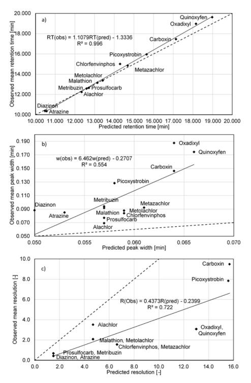
*Figure 4: Scatter plots of observed means vs. predicted values with regression lines (solid) and identity lines (scattered) for the parameters a) retention time,b) peak width and c) resolution.*
