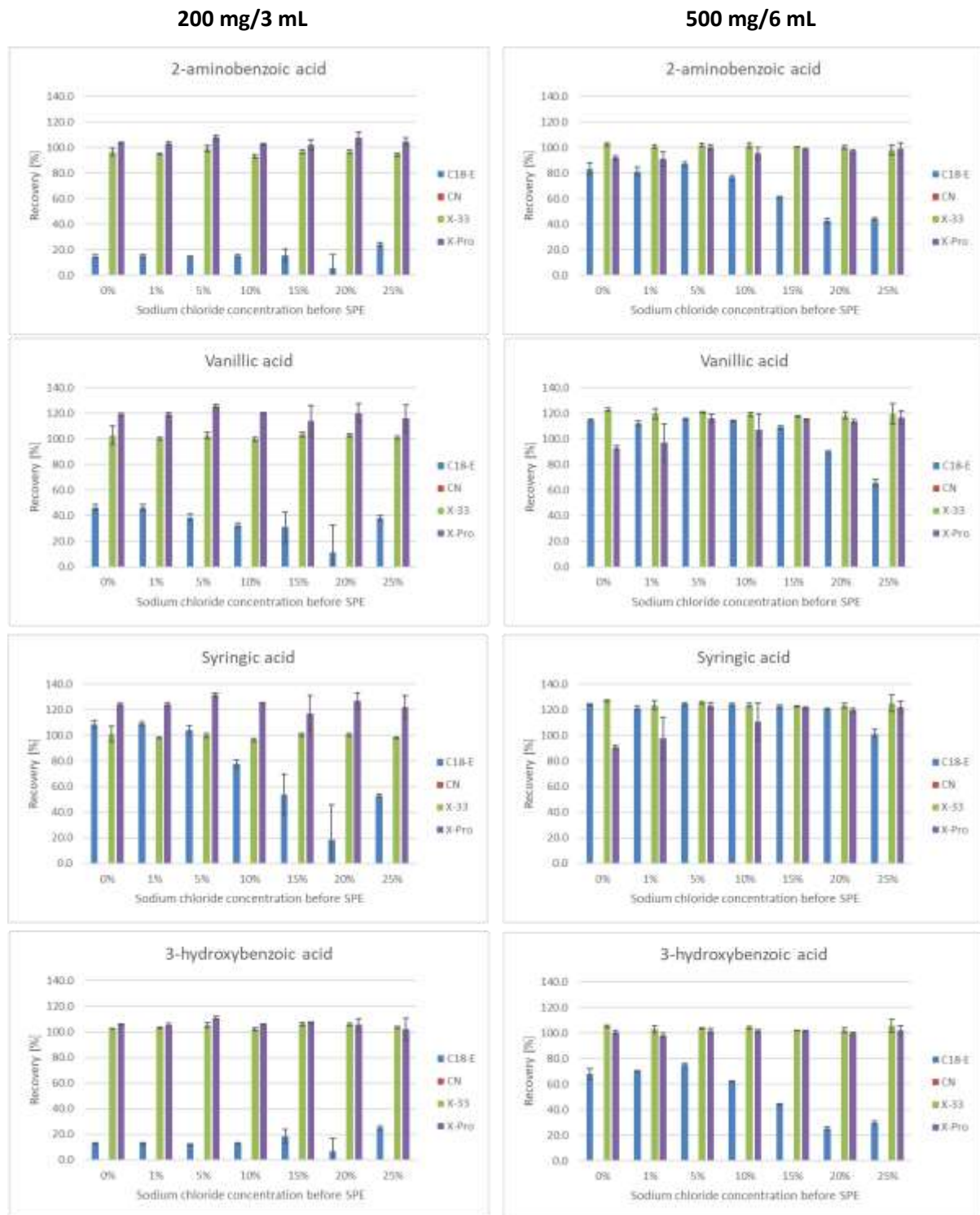
Figure 5: Recovery rates of studied compounds in the eluates for both cartridge dimensions.
